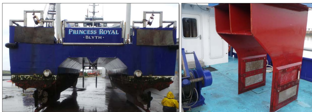
Fig. 1: The twin strut system with dynamically grown biofilms on coated surfaces deployed underneath (on the left) and deployed on board (on the right) of the RV Catamaran Princess Royal for inspection.
