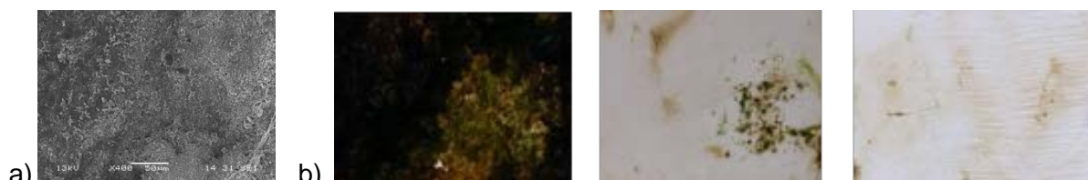
Fig. 2: MEB of hybrid paint after 24 weeks in seawater. b) Pictures of coatings without paint, with a commercial paint and with the hybrid paint after 18 months in seawater
