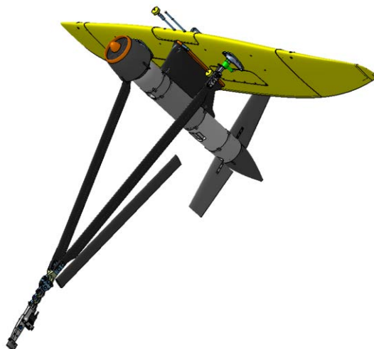
Fig. 1: Minesto's Deep Green 1/4 scale device.
