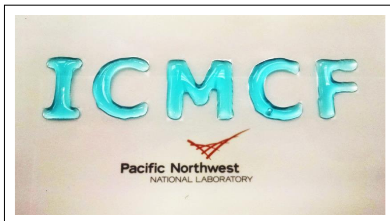
Fig. 1: A biomimetic composite coating that emulates both the superhydrophobic lotus leaf and the slippery pitcher plant repels water from the area surrounding the ICMCF lettering. This low cost sprayable coating has low surface energy and a self-healing surface.
