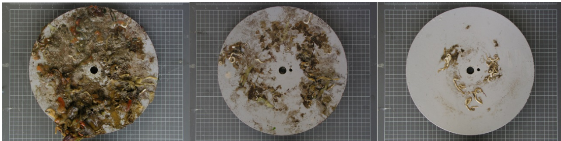
Fig. 1: Fouled FRC-coated disc (left); rotated at 700 rpm (middle); held at 1400 rpm for 15 mins (right)
