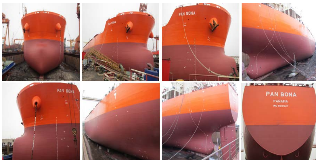
Fig. 1: Photographs of M/V "PAN BONA" after painted with low-friction AF coating
