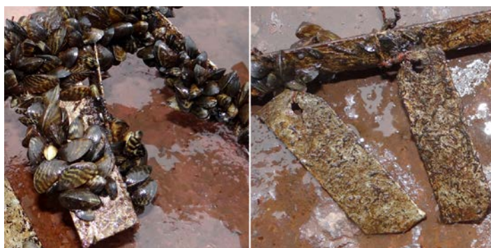
Figure 1. Painted steel bars after 228 days exposure in Dnipro River: control coating (left) and coating containing 5 wt % of PHMG molybdate (right).
