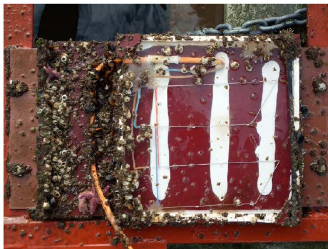
Fig. 1: ~30x30cm sample, virtually spotless after 3 month immersion at sea in high fouling conditions. The test surface outside of the active area is completely covered in barnacles.
