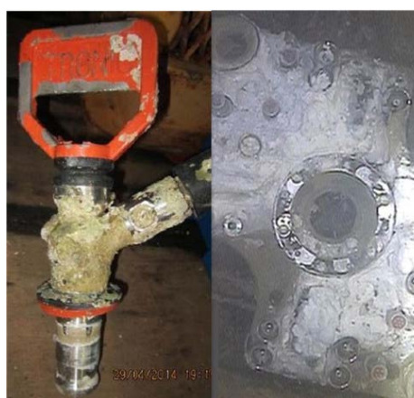
Fig. 4: Calcareous Deposits on EFL and SCMMB
