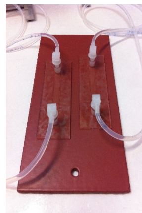
Fig. 1: Sticky-slides attached to test-surface.
